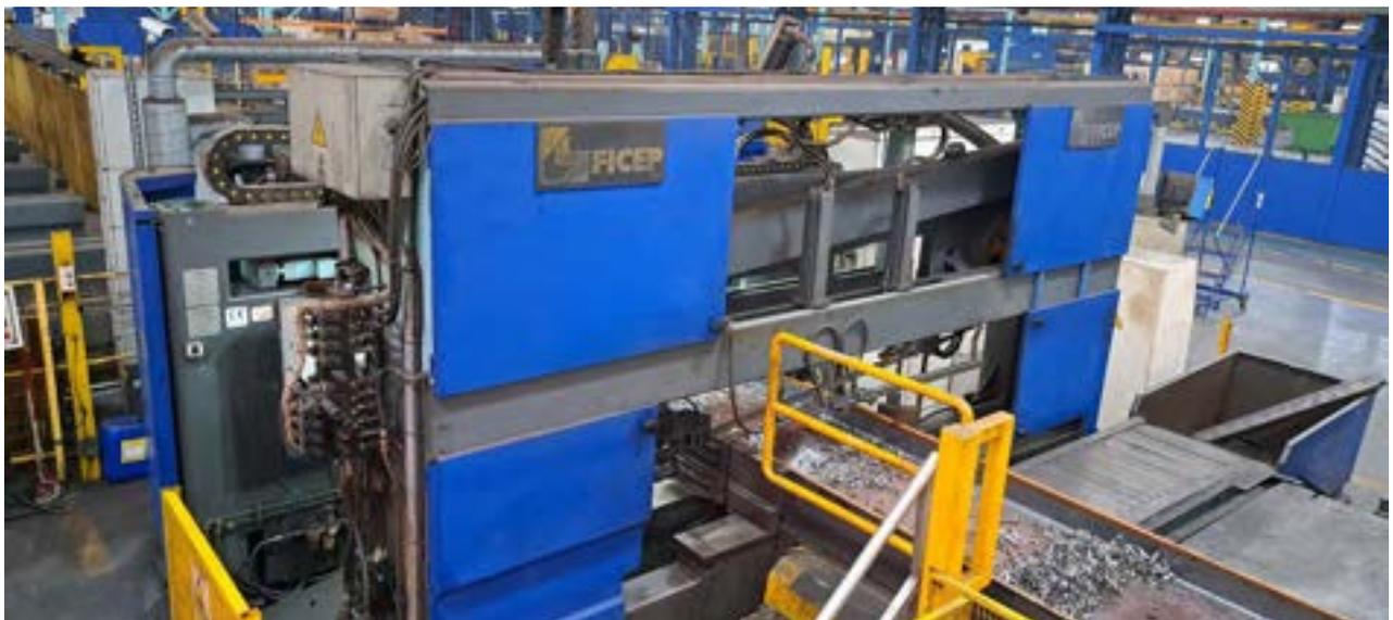
Saw drill 18m out feed and transfer:
