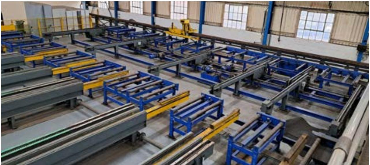
**ONE FICEP MODEL "1261 TT" AUTOMATIC THERMAL COPING MACHINE FOR BEAMS equipped with a Model FENICE 5+1 axes CNC Control System, consisting of:**
