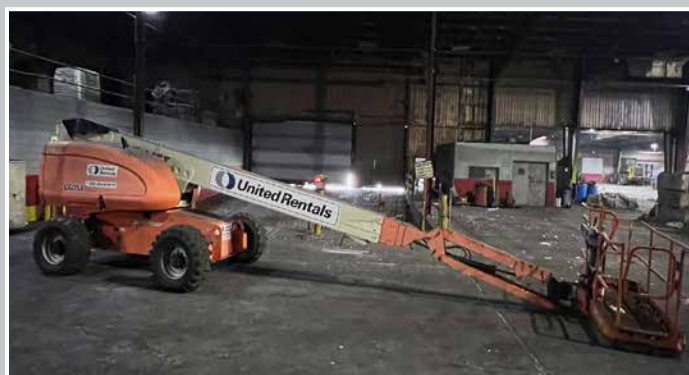
JLG 660SJ Boom Lift
