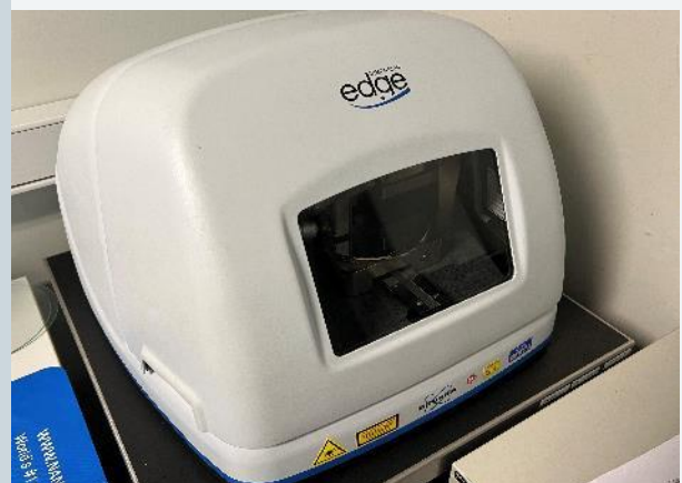
BRUKER DIMENSION EDGE ATOMIC FORCE MICROSCOPE- AFM, DOM 2013
