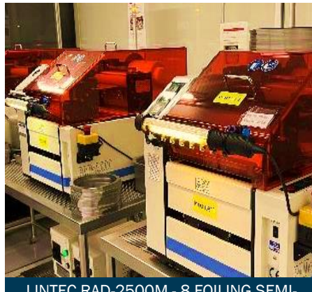
LINTEC RAD-2500M - 8 FOILING SEMI-AUTOMATIC WAFER MOUNTING SYSTEMS
